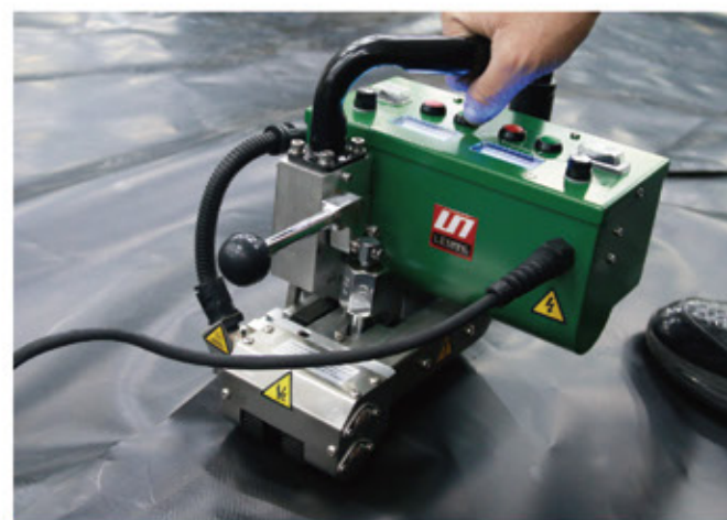
HDPE(1.5mm) 膜材焊接 LST-GM1
